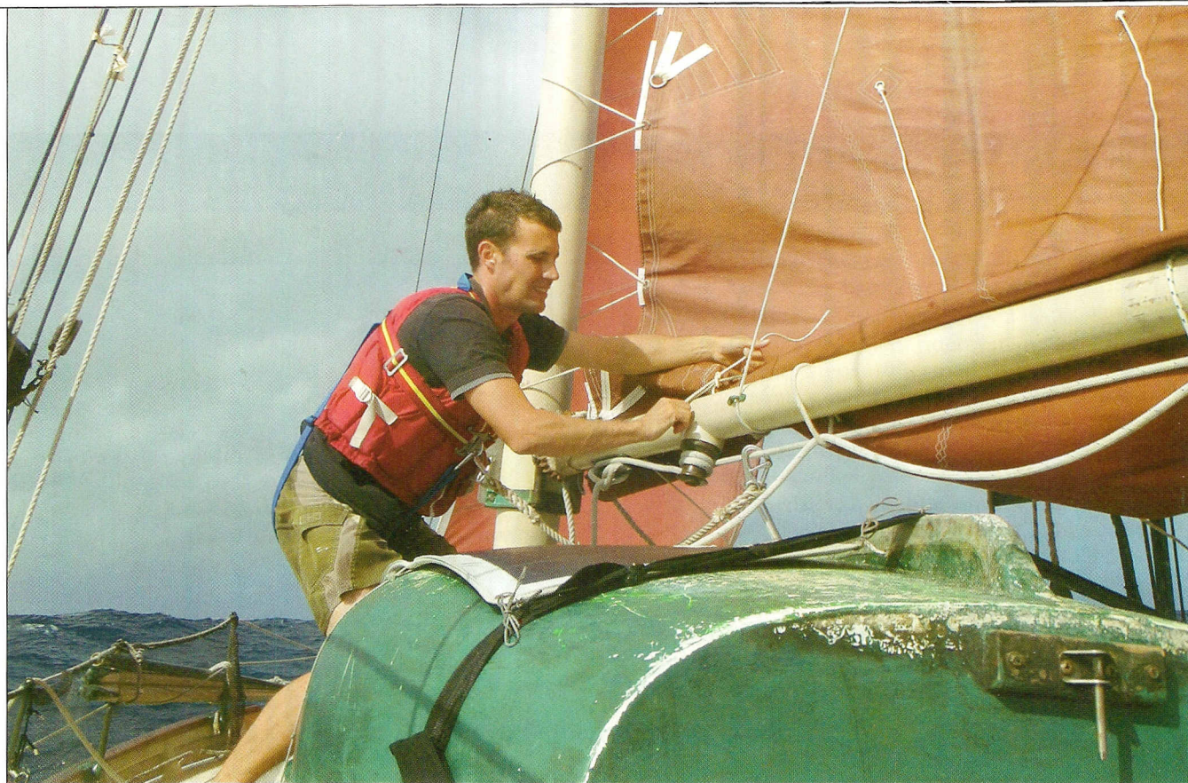
Halabisky begins tying in VIXEN's reef points (see step 5, following page). Note that, so as to not stress the sail, the line passes around the sail only, and not the boom.
