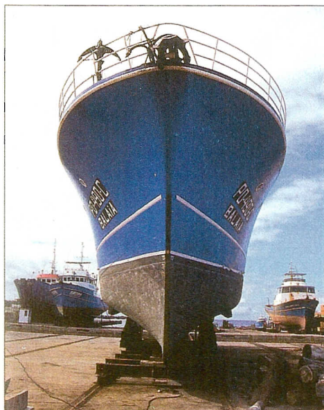
Left: The flared bow and narrow entry is typical of the Azorean fishing boat. Right: the Perola dos Açores on her launching day.
