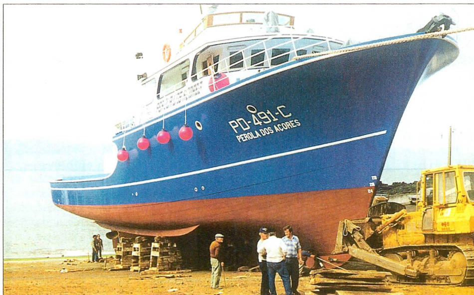
Left: The flared bow and narrow entry is typical of the Azorean fishing boat. Right: the Perola dos Açores on her launching day.
